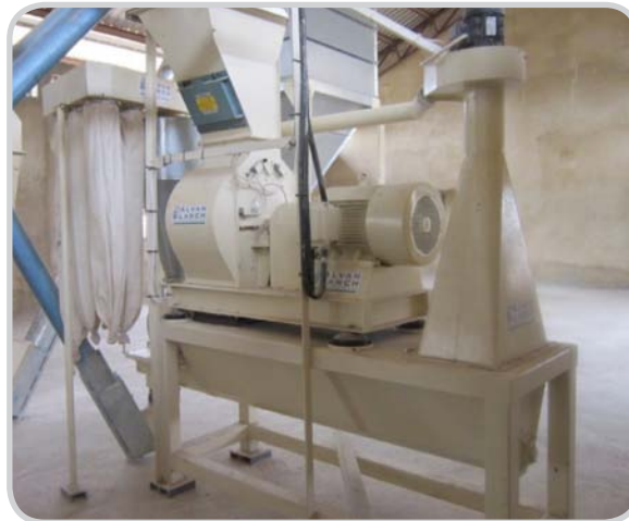
► Hammermill, fan assisted gravity discharge, with auger feeders for grain and oilcake
