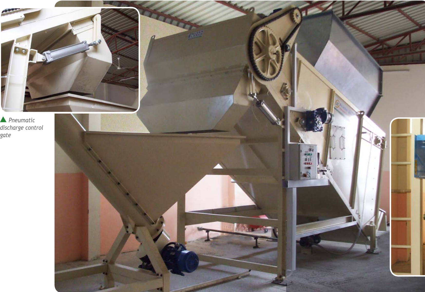
◀ Front end of the mixer - with discharge via screw conveyor to sacking hopper
