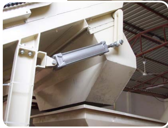
▲ Pneumatic discharge control gate
