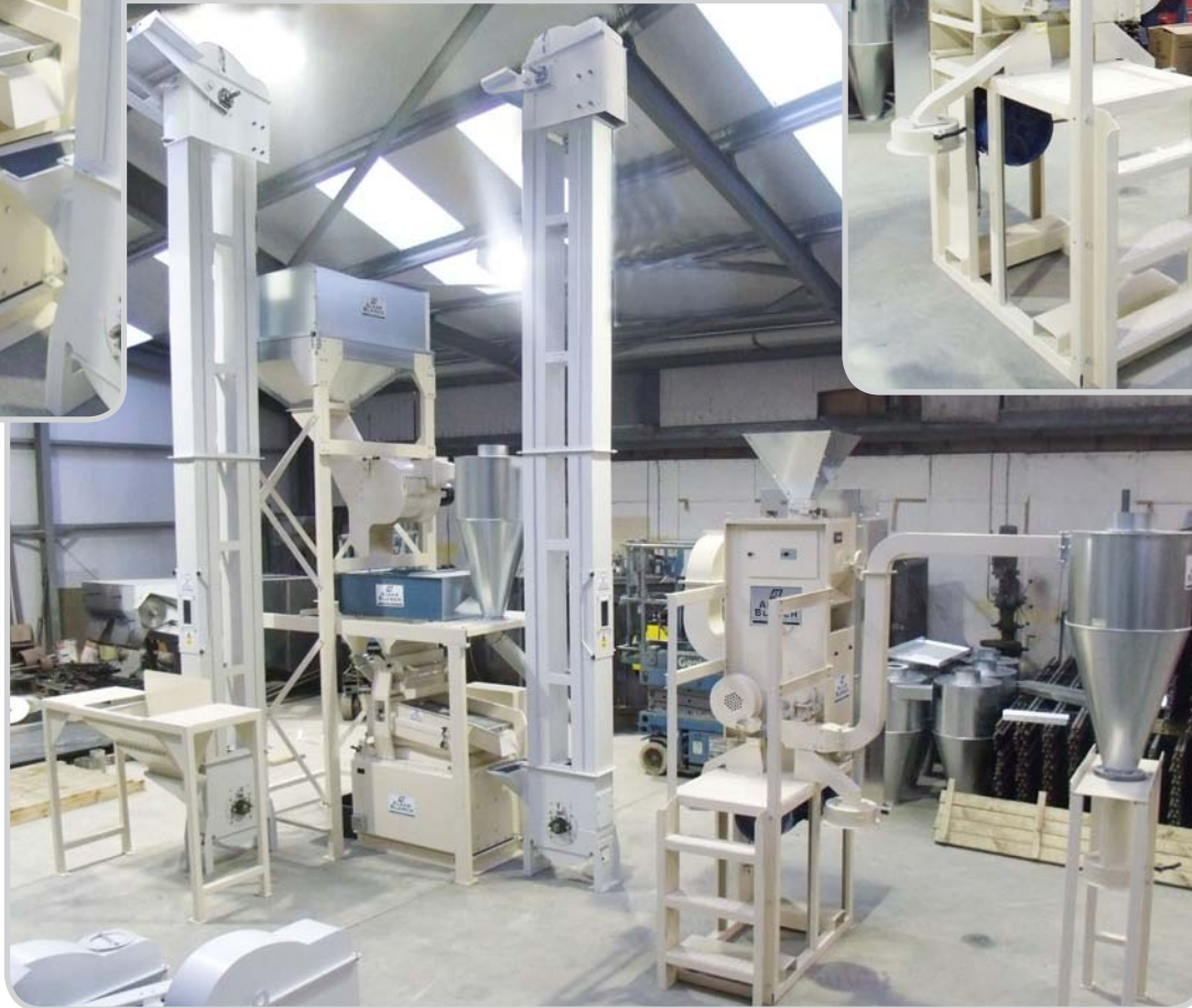
▼ The complete system - from reception and precleaning on the left to rice milling and sacking on the right
