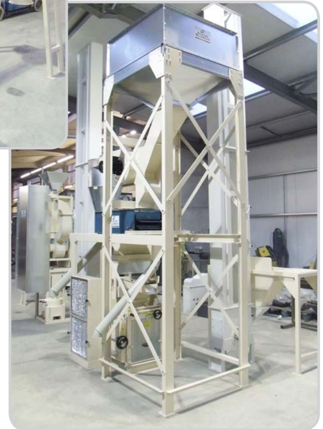
▼ Reception elevator with bag tip hopper feeding to hopper over Aspirator and Precleaner
