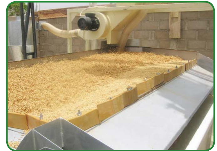
▶ Gravity Separator in the process of being set up during test run.
