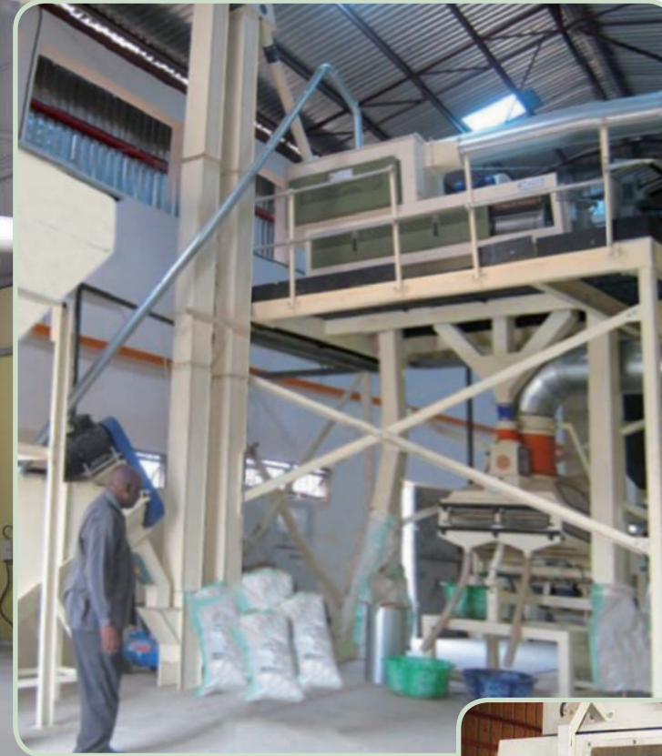
▼ The high performance rotary cleaner positioned on high platform above the destoner.
